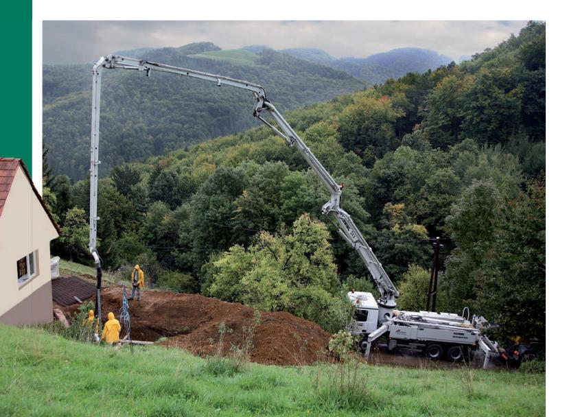
The basic substructure of this concrete pump as well is SCHWING's own anti-torsion frame, which transmits the outrigger forces directly to the corner points of the frame when the outriggers are deployed. Compared to other concepts of trestle frames, this design ensures absolutely smooth operation during pumping – particularly at the rear.
