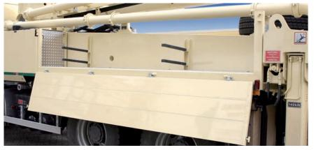
The hinged sideboard with the hose storage allows safe and operator friendly stowing of accessories and 3m long hoses or pipes.
